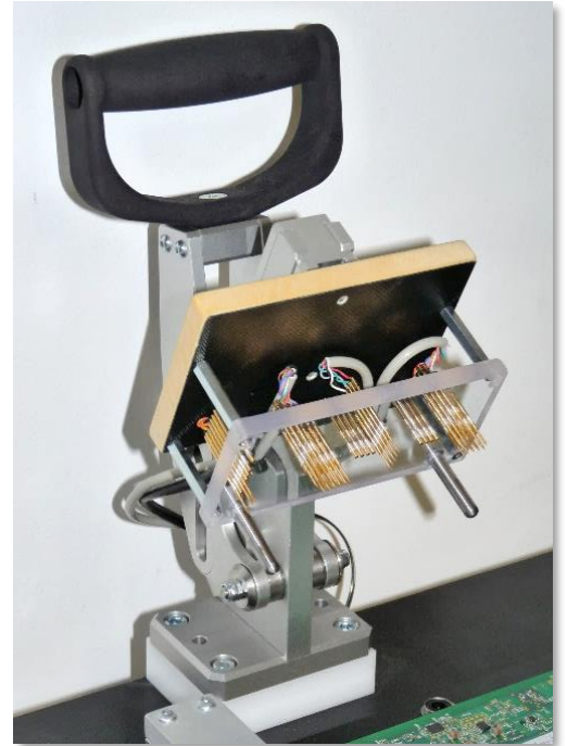
Application example: contacting of test points from above
