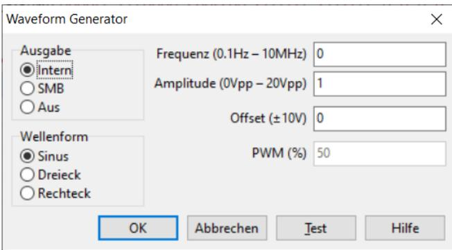
Dialog box to control the WFG2 card. Pulse width modulation PWM is only possible in the presence of square wave signals.
