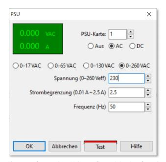
If a transformer board is configured in the Guardian hardware configuration, this dialog box controls both the PSU board and the TRF board. In AC mode, a selection of 4 voltage ranges is displayed. The variable for the current limit relates to the PSU board. This extension is included in WinGuard Version 6.10 and above.
