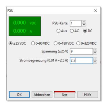
This figure displays the dialog box in DC mode. When the range ±25VDC is selected, the PSU voltage only passes through the TRF board. For other ranges, the rectified transformer output is output. More information on this process can be found in the WinGuard manual.
