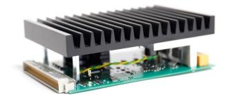
The PSU board features a four-quadrant amplifier and can generate voltages in the range of  $\pm 25V$ . The integrated A/D converters can be used to measure the output current and voltage. As the output is potential-free, two boards can be connected in series without any issues in order to double the output voltage to  $\pm 50V$ . Sense inputs are provided to compensate for the voltage drop in the connecting cables to ensure a precise power supply for the assemblies under test.
