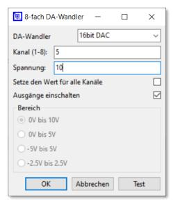
This dialog box can be used to enter a voltage for channels 1 to 8. The 9 cut-off relays are controlled with the 'Switch Off Outputs' check box. For the 16-bit variant, the 4 voltage ranges are omitted due to the higher resolution.
