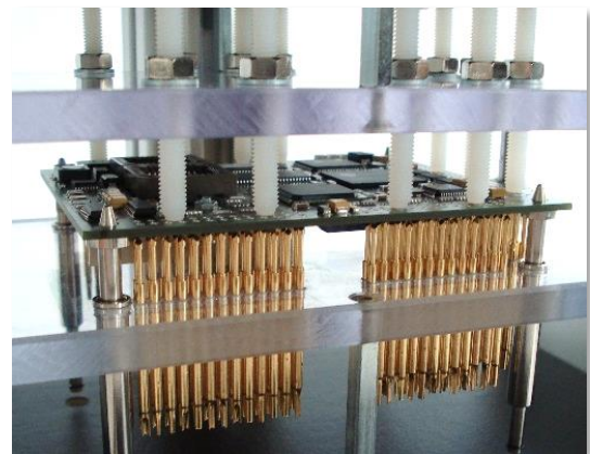
Application example 2 DUT with spring contact pins and hold-down pins
