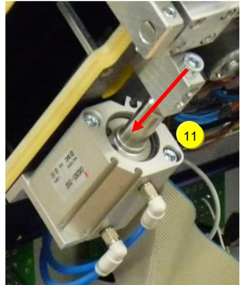
*Image 4 compressed air cylinders of pull-down mechanism*
