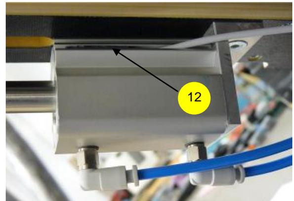
*Figure 5 sensor on pneumatic cylinder*
