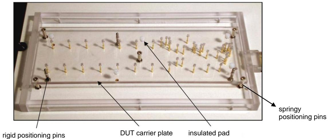
*Figure 2 carrier plate for the test specimen above the probe carrier plate*
