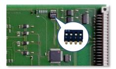
1 indicates switch position ON 0 indicates switch position OFF
