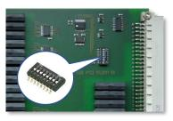
The board address is configured with a 8-pin DIP switch. The WinGuard supports up to 16 MSU boards; the base address is 128 Standard configurations are 48x2, 96x2, 192x2 or 48x4 measurement channels.
