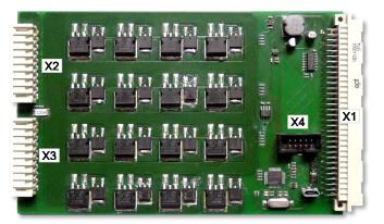
The PLD2 board includes 16 N-channel power MOSFETs, type VNB14NV04. The semiconductor switches are equipped with extensive, integrated protective circuits and a low  $R_{DS(ON)}$ . The board is suitable for switching voltages up to 40VDC and loads up to 5A against the GND system. The firmware contains a clock generator and a software-based resettable fuse for the entire current to provide protection against surges.
