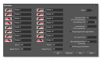
WinGuard controls the PLD2 board with this dialog box. On the left-hand side of the dialog box there are two columns with control elements for each of the board's outputs. Descriptions can be added for the outputs in the text fields.
